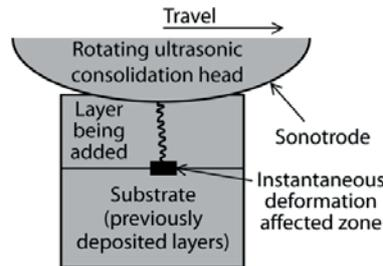
**Ultrasonic consolidation (UC)**—One of the newest additive manufacturing technologies, patented by an American company called Solidica and in development by Solidica and the Edison Welding Institute (Slattery 2011). This process uses metal foils held together under pressure, combined with ultrasonic vibrations that create a weld between layers of foil, which are then machined to the desired shape (Domack and Baughman 2005).
