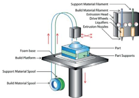
**Fused deposition modeling (FDM)**—This process uses hot nozzles to extrude polymeric material into position, using one nozzle to extrude support material and a second to extrude the part.
