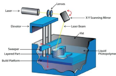
**Stereolithography**—This process makes use of photo-curable plastic resins that are treated by UV laser to become solid or gel-like and is most often used for prototyping (Hopkinson 2010).
